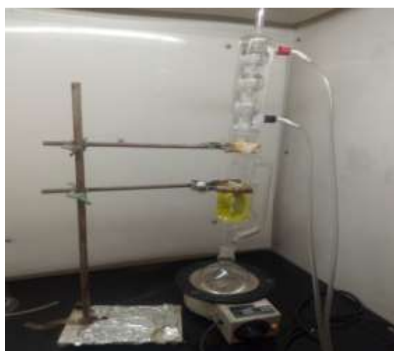
Figure 1: Extraction of oil Neem leaves using Soxhlet extraction method
